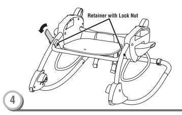
• Fit a retainer with lock nut onto the end of a screw and to the inside of a side rail. Tighten the screw using the assembly tool. Turn the tool clockwise to tighten.
